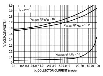
Figure 1. "Saturation" and "On" Voltages
