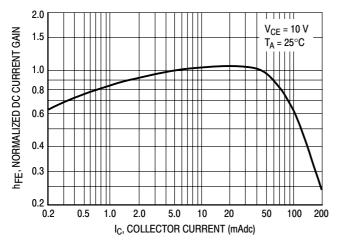
Figure 1. Normalized DC Current Gain
